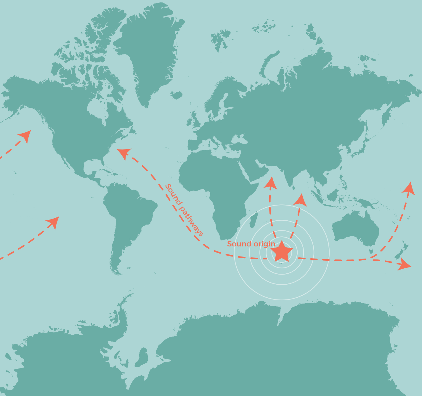
Figure 2. Low frequency sound can travel for hundreds or even thousands of kilometres, especially when travelling in deep ocean channels. 4 These channels occur as a result of changes in water temperature (surface water changes with outside temperature while deeper water maintains more constant temperatures), differences in salinity, and increased pressure with depth, which compresses water molecules. The red arrows show the transmission distance of a tone that was broadcast at less than 100 Hz.
