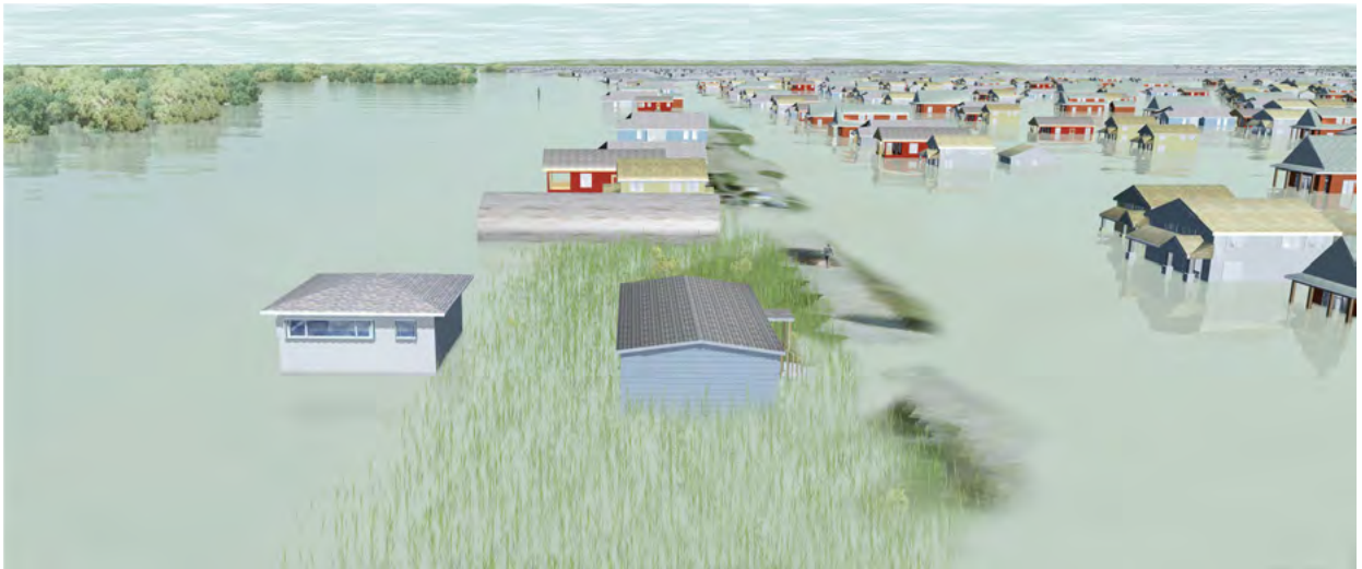
Figure 12. Breach of the Ladner Dike with a projected 1.2 metres of sea level rise by 2100, plus storm surge, plus high tide. Future high water level of 4.16 metres, Delcan 2011. Source: Delta RAC, CC-BY-NC-ND
